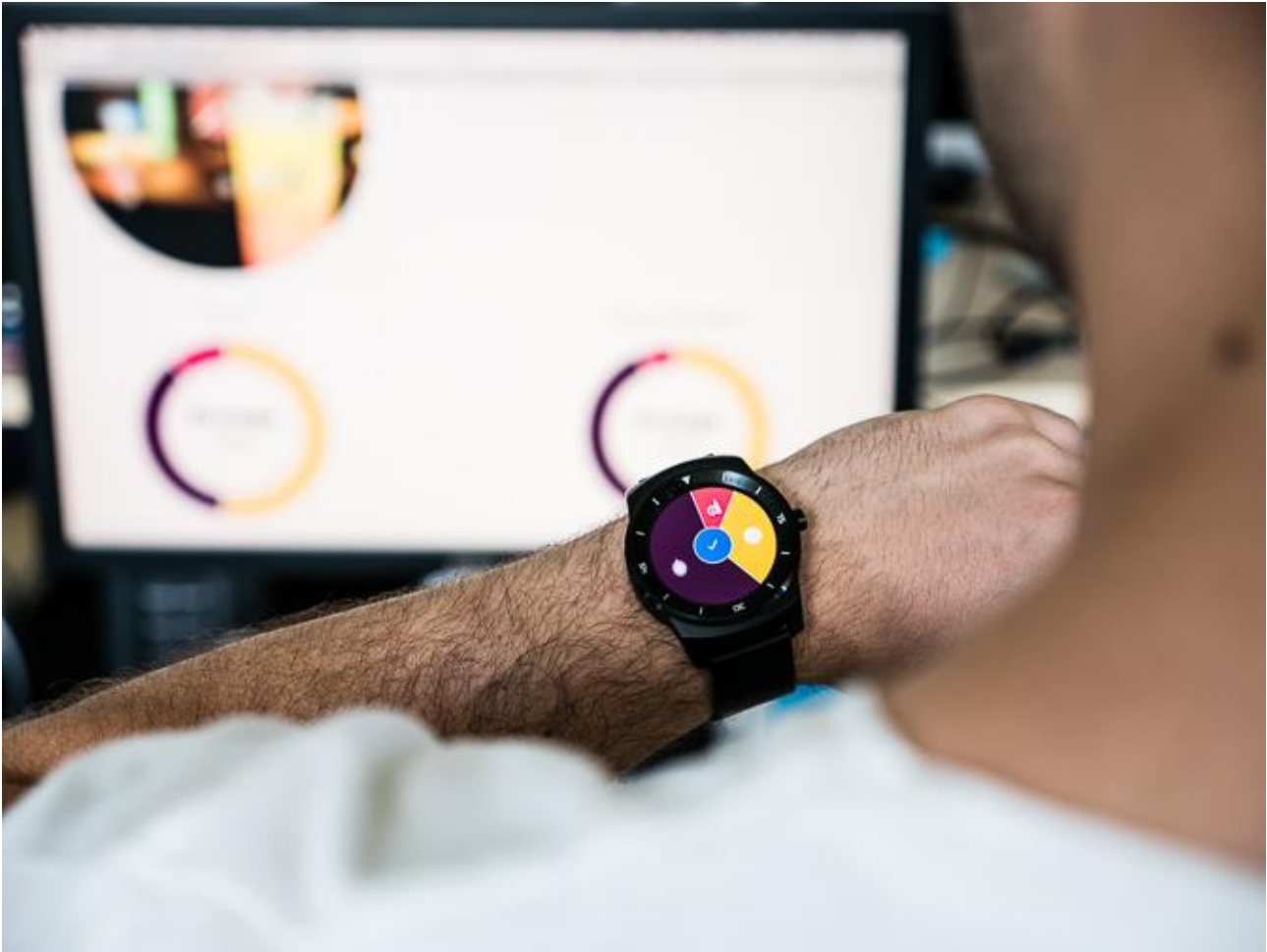
Figure 3: Hands-free interaction with notifications and production processes in the manufacturing environment using smartwatches (Gottwalles, 2016)
