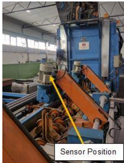
Figure 9: Vibration sensor position at Bossi machine
